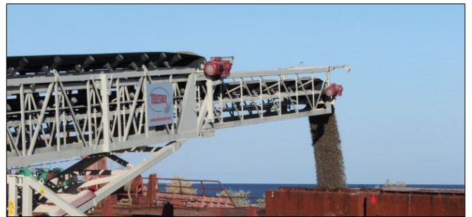
Heavy Duty lattice frame design
